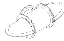
A standard Sidepower sternthruster tunnel with the add-on cowls for shallow installation.
