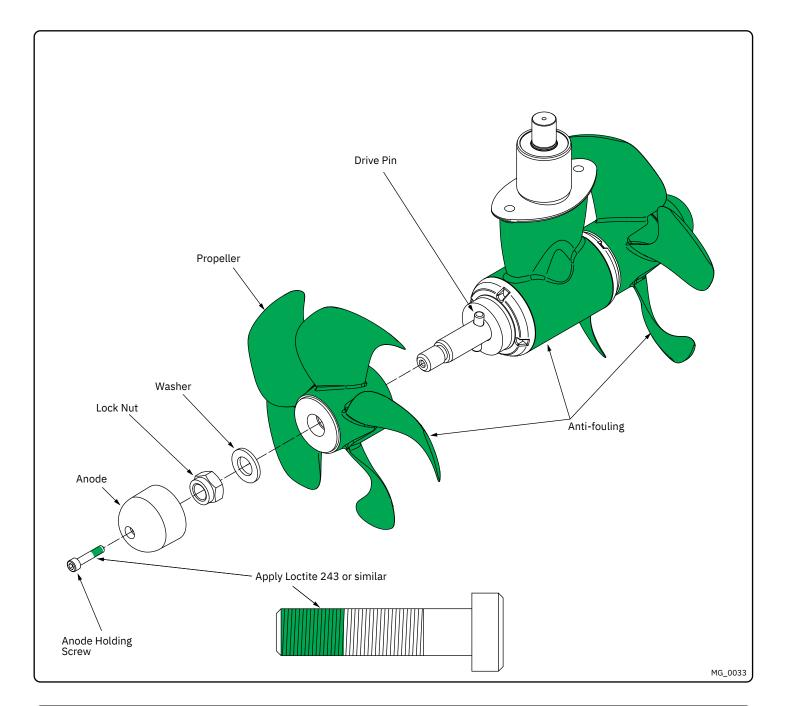
Propeller Installation MC\_0264
