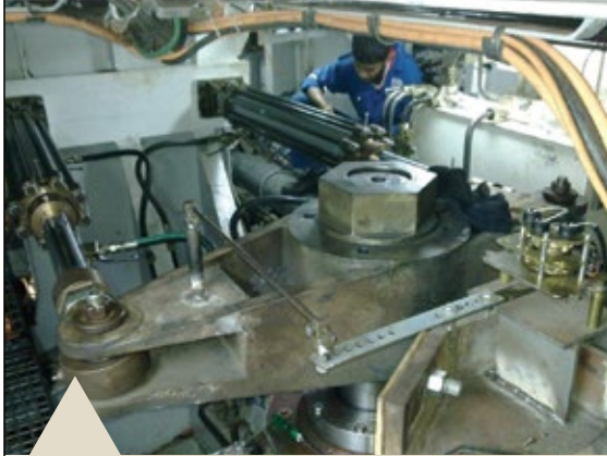
A 9-ton meter steering arrangement for a twin screw tug with electronically synchronized rudder (no mechanical tie bar to the second rudder).
