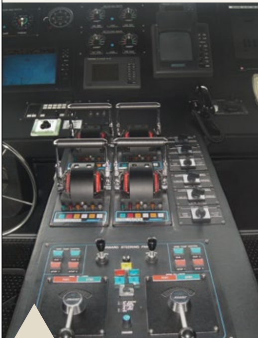
A 4-engine electronic propulsion control with Kobelt steering gear and rudder angle indicators. The complete package is provided by Kobelt.
